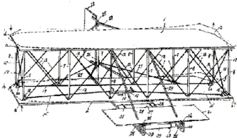
Fig 5: the Wright brothers patented drawing of aeroplane.
