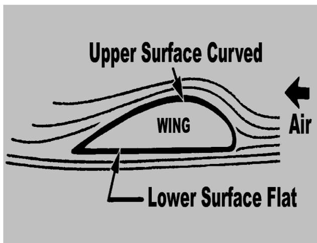
Fig 7: Cross section of a plane wing
